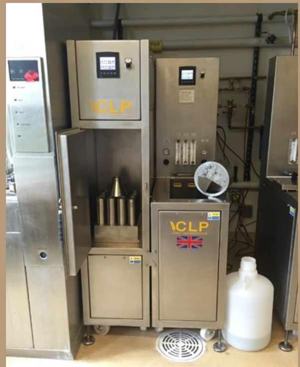
Combi malter: Kiln on left, steep/germ on right
