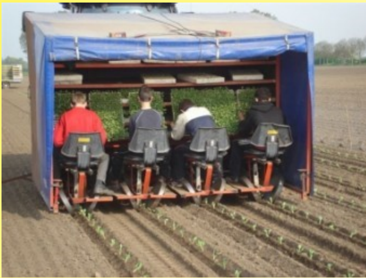
Small- to mid-sized vegetable growers can use planting aids, such as this Brassica transplant planter.
